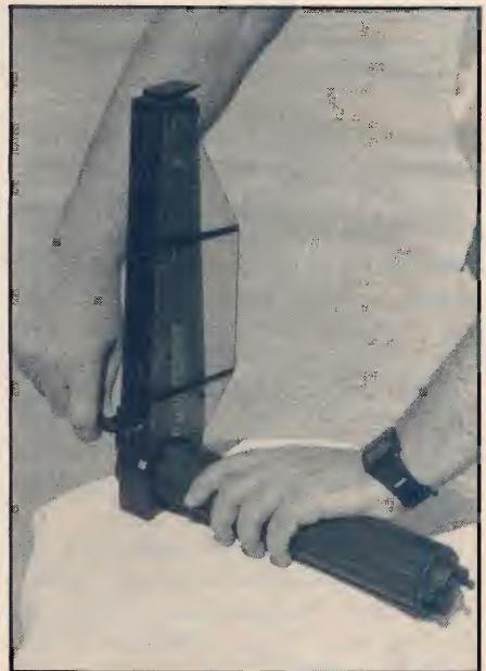
The M-900 magazine speed loader permits the loading of a magazine in as little as 30 seconds.
